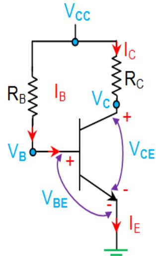
$$I_B = \frac{V_{CC} - V_{BE}}{R_B}$$
