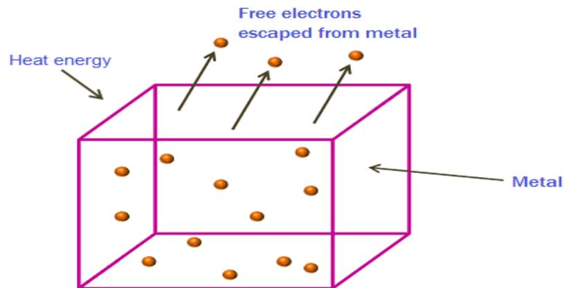
The process of electron emission from a metal surface by supplying thermal energy to it is known as thermionic emission.
