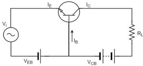
For a transistor to be operated as a faithful amplifier, the operating point should be stabilized.
