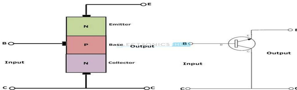
The ratio of change in emitter current ( $\Delta I_E$ ) to the change in base current ( $\Delta I_B$ ) is known as **current amplification factor** in common collector (CC) arrangement i.e.  $\gamma = \Delta I_E / \Delta I_B$
