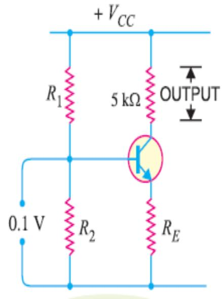
Due to transistor action, a much larger ( $\beta$  times the base current) a.c. current flows through the the load  $R_c$  in the output circuit. Since the value of load resistance  $R_c$  is very high, a large voltage will drop across it.
