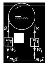
Here we have a system of particle connected between themselves and so constrained that each particle can have only a rectilinear motion.
