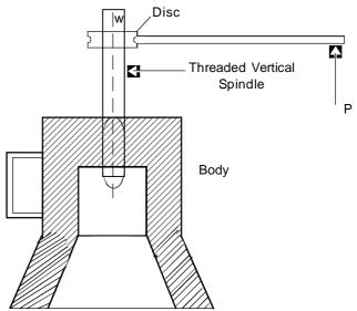
A Simple Screw Jack consists a vertical threaded spindle. The treaded portion of the spindle passes throught a nut cut in the body of the Screw Jack.
