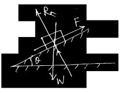
Consider a block of weight 'W' resting on a rough inclined plane (angle)
