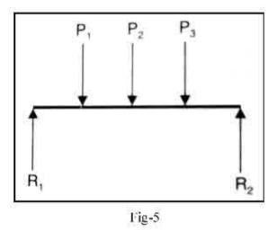
In this system, the lines of action of all the forces lie in the same plane and are parallel to each other but may not have same direction as shown in the figure.
