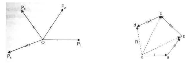
If the forces  $P_1, P_2, P_3$  and  $P_4$  acting simultaneously on a particle be represented in magnitude and direction by the sides *oa*, *ab*, *bc* and *cd* of a polygon respectively, their resultant is represented by the closing side '*do*' in the opposite direction as shown in the figure.
