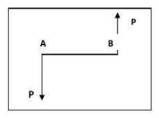
The effect of couple acting on a rigid body is to rotate it without moving it as a whole.
