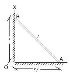
displacement – time, velocity-time and acceleration-time equations for the vertical motion of the end B of the bar.
