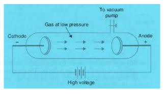
The rays were found to cause fluorescence on the glass tube where they fall. **Sir J. J. Thomson** made an extensive study on the properties of cathode rays.
