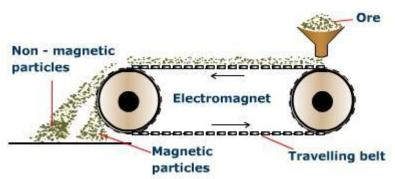
method a belt is tied over two rollers of which one is made up of magnet. Pulverized ore is added over the belt through a hopper. The pulverized ore move towards the magnetic pulley along with the rotating belt. The non-magnetic impurities fall directly below the magnetic pulley while the magnetic ore form a separate heap due to the influence of the magnetic field.
