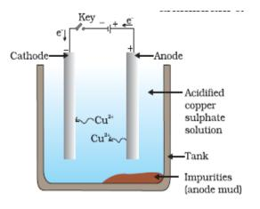
• The electrodes are connected to an external source of emf (battery). The electrode which is connected with the positive end of the battery is called **anode** and the electrode which is connected to the negative end is called **cathode**.
