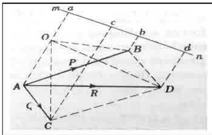
In the plane of action of forces , we take any line  $mn$  perpendicular to the line OA joining the moment center with the point of concurrence of the forces and construct the perpendiculars  $Aa, Bb, Cc$  and  $Dd$  , as shown in figure.
