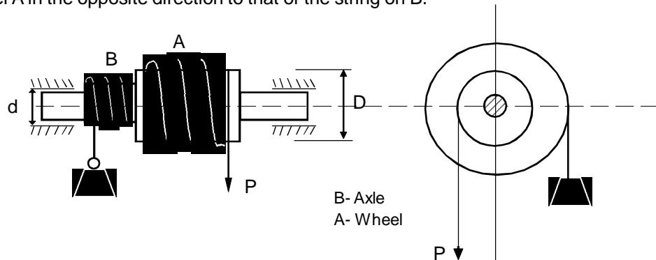
**Fig 2.1 Simple wheel and axle**
