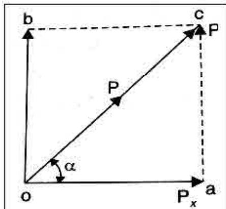
Let  $P_x$  is the component of force  $P$  in the direction  $oa$  making an angle ' $\alpha$ ' with the direction  $oc$ .
