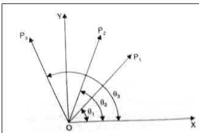
The resolution of  $P_1$  in the direction OX is  $P_1 \cos \theta_1$ , and in the direction OY is OX is  $P_1 \sin \theta_1$ .
