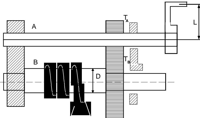
Fig 2:3 Single Purchase Crab Winch. In a Single Purchase Crab Winch, a rope is fixed to the drum and wound. A spur gear (B) is mounted on the load drum. Another pinion A is geared with (B) and connect to effor wheel.
