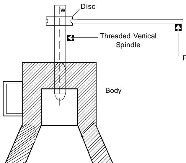
A Simple Screw Jack consists of a vertical threaded spindle. The threaded portion of the spindle passes through a nut cut in the body of the Screw Jack.
