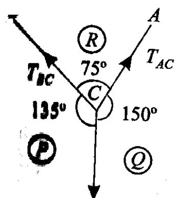
According to the system of forces and the above figure, we find that angle between  $T_{AC}$  and ISN is  $150^0$  and angle between  $T_{BC}$  and 15 N is  $135^0$ .
