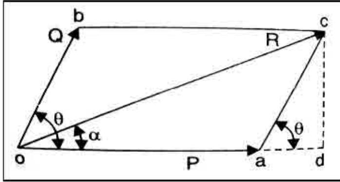
From the geometry of the figure  $\angle CAD = \theta$ ,  $AC = Q$ .
