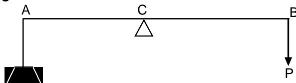
When the effort P is withdrawn the end A will go down wards raising the end B upwards. We say that the lever is reversible.
