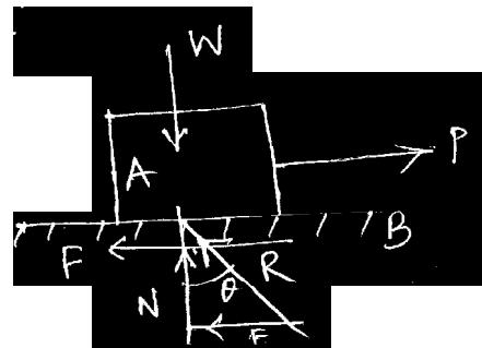
Let  $R$  be the resultant reaction between normal reaction and force of friction acts at angle  $\theta$  to the normal Reaction.  $\theta \rightarrow$  Angle of friction.
