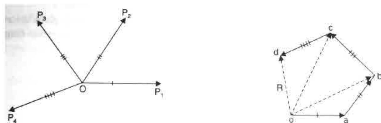
If the forces  $P_1, P_2, P_3$  and  $P_4$  acting simultaneously on a particle be represented in magnitude and direction by the sides  $oa, ab, bc$  and  $cd$  of a polygon respectively, their resultant is represented by the closing side ' $od$ ' in the opposite direction as shown in the figure.
