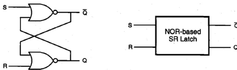
Fig 6.8 (Gate-level schematic and block diagram of the NOR-based SR latch.)
