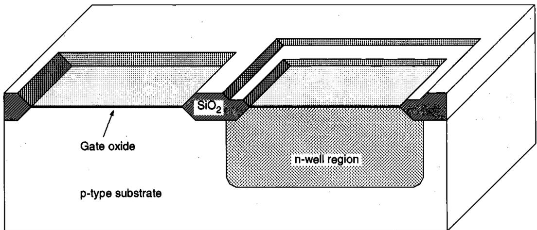
Following the creation of the n-well region, a thick field oxide is grown in the areas surrounding the transistor's active regions, and a thin gate oxide is grown on top of the active regions
