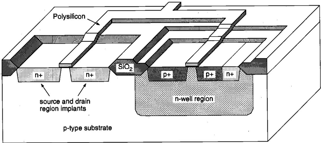
Using a set of two masks, the n+ and p+ regions are implanted into the substrate and into the n-well, respectively.
