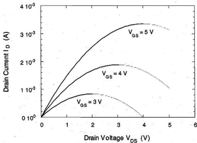
The drain current-drain voltage curves shown above reach their peak value for  $V_{DS} = V_{GS} - V_{T0}$ . Beyond this maximum, each curve exhibits a negative differential conductance, which is not observed in actual MOSFET current-voltage measurements (section shown by the dashed lines). We must remember now that the drain current equation (4) has been derived under the following voltage assumptions,
