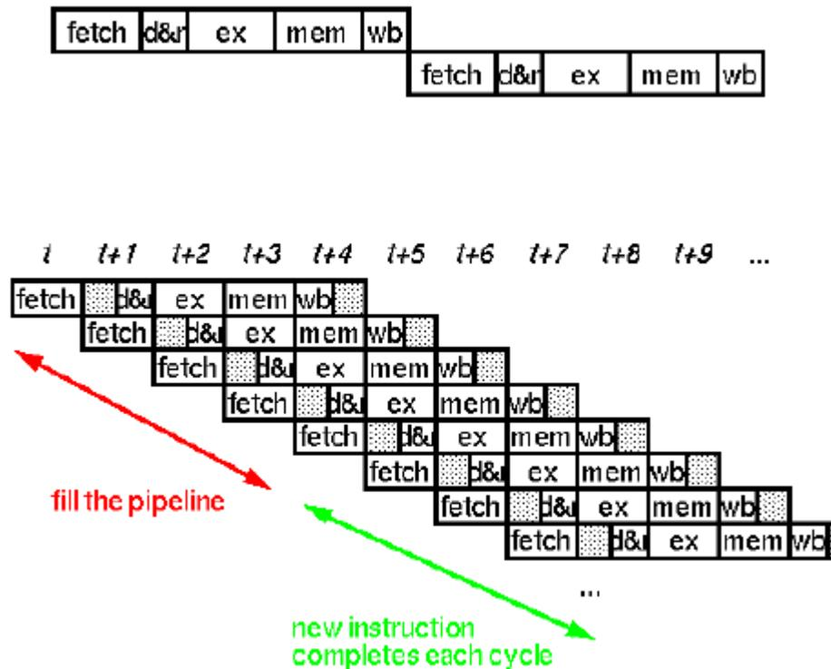
pipeline hazards is of three types 1. structural, 2. data, 3. Control place a “soft limit” on the number of stages increase instruction latency (a little) write & read pipeline registers for data that is computed in a stage time for clock & control lines to reach all stages all stages are the same length which is determined by the longest stage stage length determines clock cycle time.
