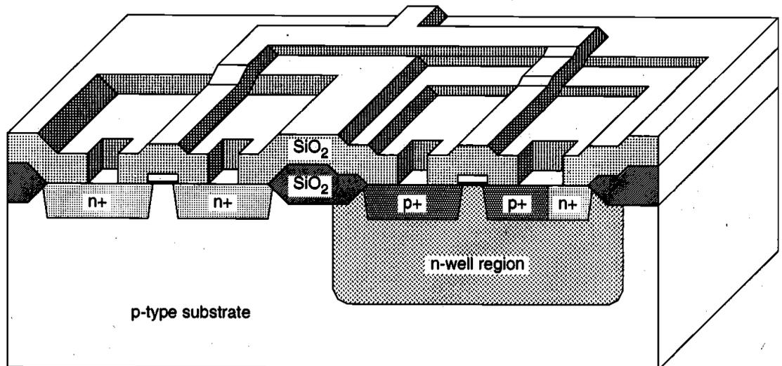
An insulating silicon dioxide layer is deposited over the entire wafer using CVD. Then, the contacts are defined and etched away to expose the silicon or polysilicon contact windows. These contact windows are necessary to complete the circuit interconnections using the metal layer,
