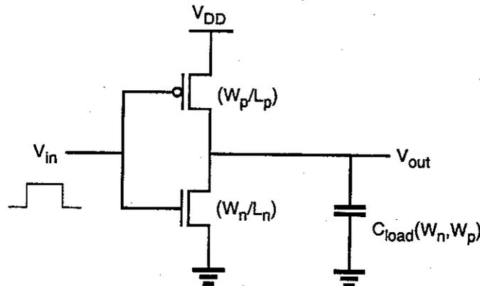
$$\left(\frac{W_n}{L_n}\right) = \frac{C_{load}}{\tau_{PHL}^* \mu_n C_{ox} (V_{DD} - V_{T,n})} \left[ \frac{2V_{T,n}}{V_{DD} - V_{T,n}} + \ln \left( \frac{4(V_{DD} - V_{T,n})}{V_{DD}} - 1 \right) \right]$$
