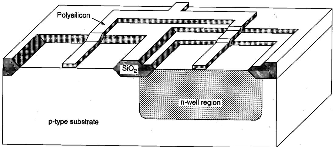
The polysilicon layer is deposited using chemical vapor deposition (CVD) and patterned by dry (plasma) etching. The created polysilicon lines will function as the gate electrodes of the nMOS and the pMOS transistors and their interconnects.
