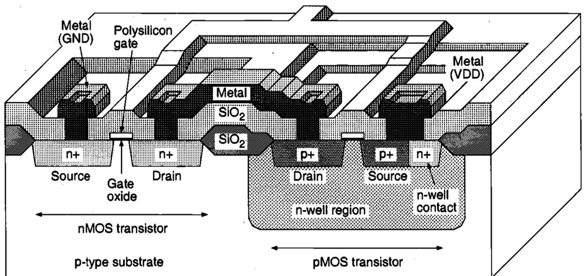
The composite layout and the resulting cross-sectional view of the chip, showing one nMOS and one pMOS transistor (in the n-well), and the poly-silicon and metal interconnections. The final step is to deposit the passivation layer (for protection) over the chip, except over wire-bonding pad areas
