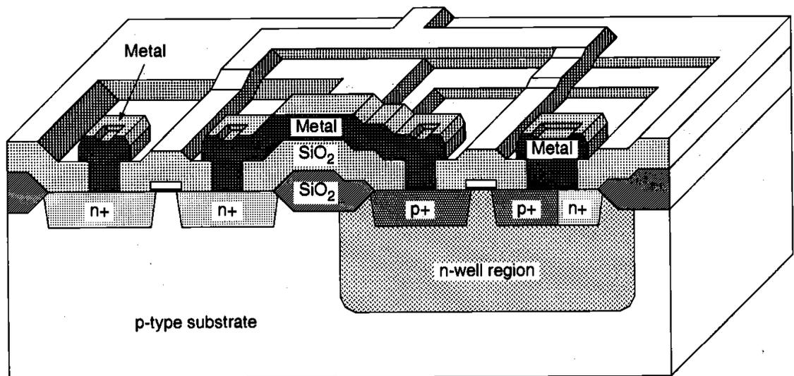
Metal (aluminum) is deposited over the entire chip surface using metal evaporation, and the metal lines are patterned through etching. Since the wafer surface is non-planar, the quality and the integrity of the metal lines created in this step are very critical and are ultimately essential for circuit reliability.
