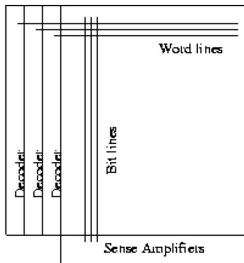
The usual layout convention is that a simple array is read out vertically. That is, a single word line, which runs horizontally, causes a row of bit cells to put their data on bit lines, which run vertically. Sense amps, which convert low-swing read bitlines into full-swing logic levels, are usually at the bottom (by convention). Larger register files are then sometimes constructed by tiling mirrored and rotated simple arrays.
