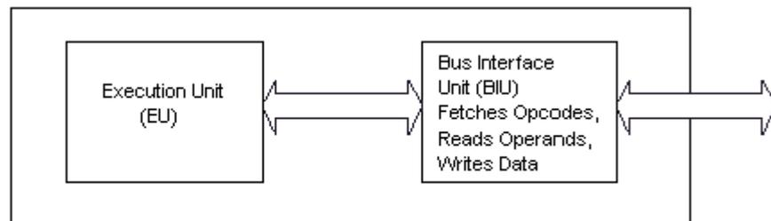
The EU receives program instruction codes and data from the BIU, executes these instructions, and store the results in the general registers. By passing the data back to the BIU, data can also be stored in a memory location or written to an output device. Note that the EU has no connection to the system buses. It receives and outputs all its data through the BIU.
