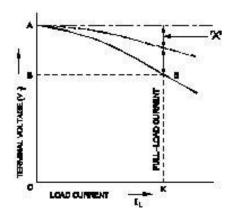
A -Full load voltage drop B- Armature voltage drop C -Armature reaction drop D- Shunt field voltage drop
