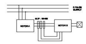
A- Cascade operation method B- Rotor rheostat control method C -Changing applied voltage method D- Injecting emf in rotor circuit method
