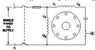
A- Permanent capacitor motor B- Capacitor start capacitor run motor C- Induction start induction run
