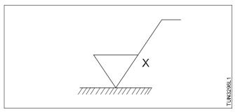
14 The surface roughness indicated by the symbol as per BIS system . What does the symbol indicate?
