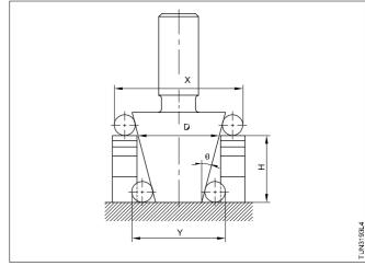
7 Formula for determining the large diameter of taper at any desired height is
