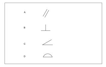
5 Name the symbol of tolerance to the surface.
