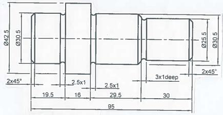
All dimensions are in mm Gen. tolerance + 0.1mm.
