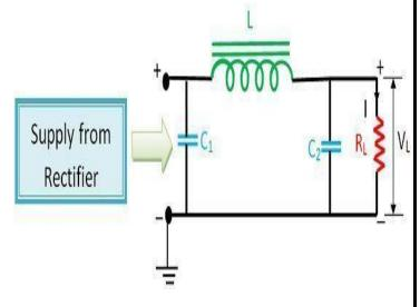
in series and another filter capacitor  $C_2$  connected across the load. The shape of the circuit diagram of this filter circuit appears like Greek letter  $\pi$  (pi) and hence the name  $\pi$ -filter.
