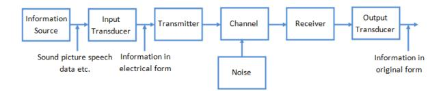
The essential components of a communication system are information source, input transducer, transmitter, communication channel, receiver and destination.
