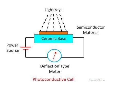
When the beam of light falls on the semiconductor material, their conductivity increases and the material works like a closed switch. The current starts flowing into the material and deflects the pointer of the meter.
