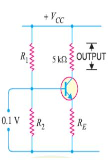
Due to transistor action, a much larger ( $\beta$  times the base current) a.c. current flows through the load  $R_c$  in the output circuit. Since the value of load resistance  $R_c$  is very high, a large voltage will drop across it.
