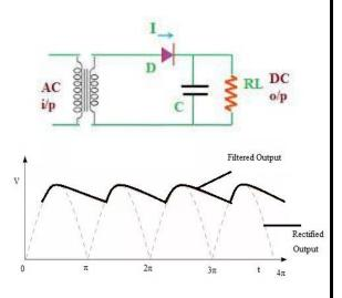
It is also called Capacitor Filter. It offers low reactance to ac &a very high reactance to the dc component. The capacitive reactance is  $X_C=1/2\pi fc$ , ford.c, f=0 Then,  $X_C=\infty$
