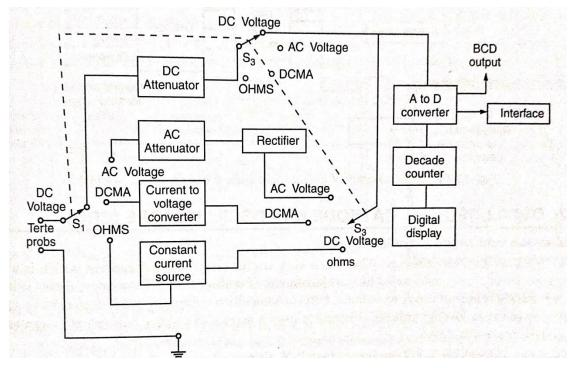
A commercial digital multimeter consist of several A to D converters, decade counters and display. It is basically dc voltmeter. In order to measure unknown current; current to voltage converter is used. An unknown current to be measured is applied to one of the input terminals of op-amp. Since input impedance of op-amp is very high; very small current can pass through it. This current passing into the op-amp can be neglected.
